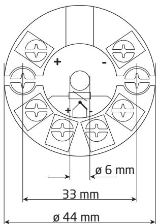
**Mounting of sensor wires**
